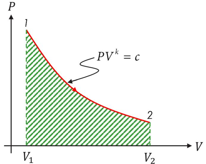
$$P = \frac{c}{V^k} ; {}_1w_2 = -\int_{V_1}^{V_2} P dV = -\int_{V_1}^{V_2} \frac{c}{V^k} dV = -c \int_{V_1}^{V_2} V^{-k} dV$$
